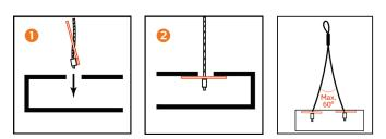
**IMPORTANT:** Maintain an angle of 60 degrees for the Luma-Lock span.
