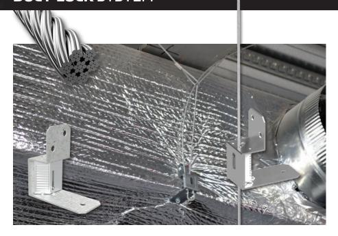
THE DUCT-LOCK SYSTEM is utilised to connect a wire rope suspension to rectangular ductwork. This allows for the suspension of ductwork without the need of using a bearer underneath. It consists of a Zip-Clip KL100 locking device and a specially shaped bracket (KV bracket) which encases the device and secures the wire suspension to the ductwork.
